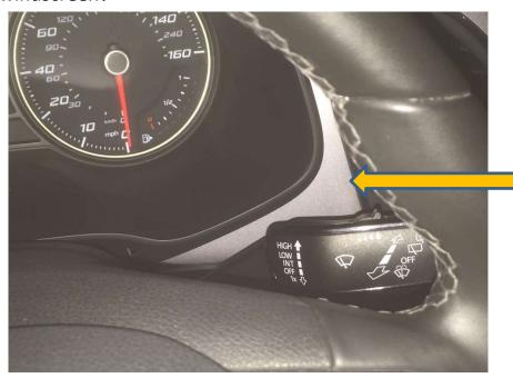
The windscreen wipers are operated on the stalk to the right of the steering column. To clean the rear window, push the stalk towards the dashboard until you hear the pump operate and deliver water to the rear screen. After operation return the stalk to the normal position.
