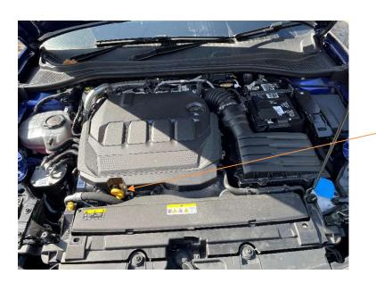
The dipstick is here, you would wipe clean, dip in the same opening and check levels as required. Replace back in the opening once completed
