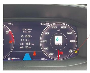
The rear fog light warning is illuminated in the right bottom corner of the digital display. N.B. this may not be the view that is active in the car.
