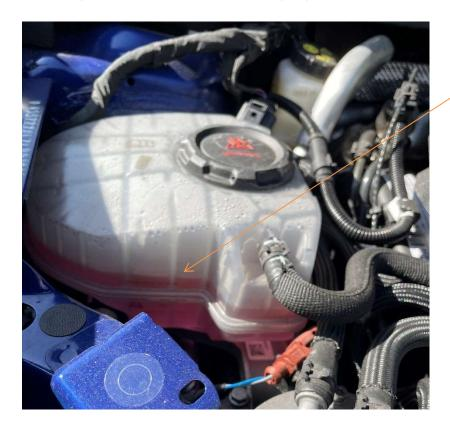
This is the engine coolant reservoir. The min and max levels are marked on the front.
