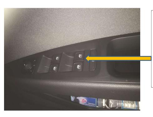
The windows are opened using the switches on the driver's door handle. There is a separate switch for each window. To open the relevant window, press the corresponding switch to open. To close the window pull the same switch up until the window closes.
