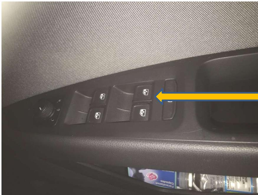
The windows are opened using the switches on the driver's door handle. There is a separate switch for each window. To open the relevant window, press the corresponding switch to open. To close the window pull the same switch up until the window closes.
