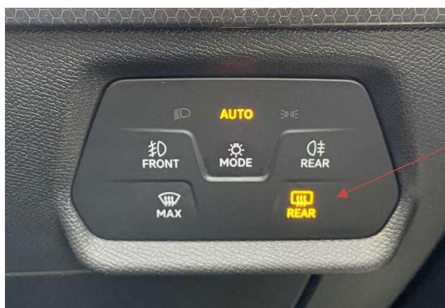
On the touch pad touch the bottom right symbol showing a heating element above the word REAR.
