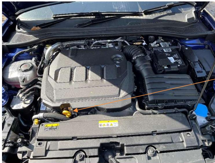
The dipstick is here, you would wipe clean, dip in the same opening and check levels as required. Replace back in the opening once completed
