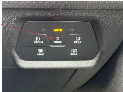
The touch panel will look like this when no lights or heating controls are active. The headlights are automatic and will come on in poor light.
