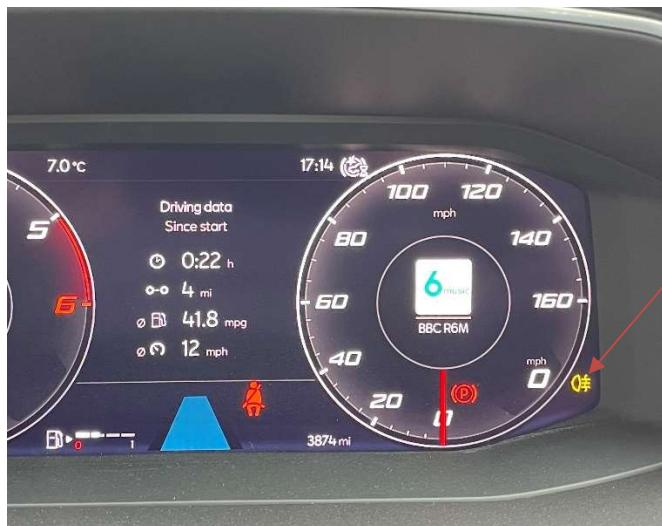
The rear fog light warning is illuminated in the right bottom corner of the digital display. N.B. this may not be the view that is active in the car.
